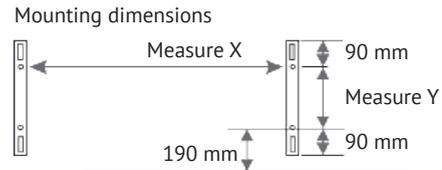
All radiators have four temperature-resistant holders, which guarantee optimum fixing of the heater. Please note the correct hanging position of the upper (marking 1) and lower (marking 2) holders on the heater.
