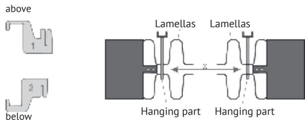
With the type-specific dimension table, you can obtain the correct positioning for the U-rails and the holders for the correct mounting and fixing of the radiator.
